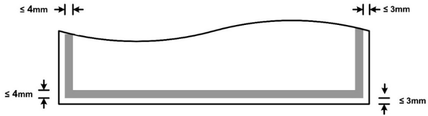
Figure 22 – Standard One-Piece Mailer – glue line requirements (not to scale)
