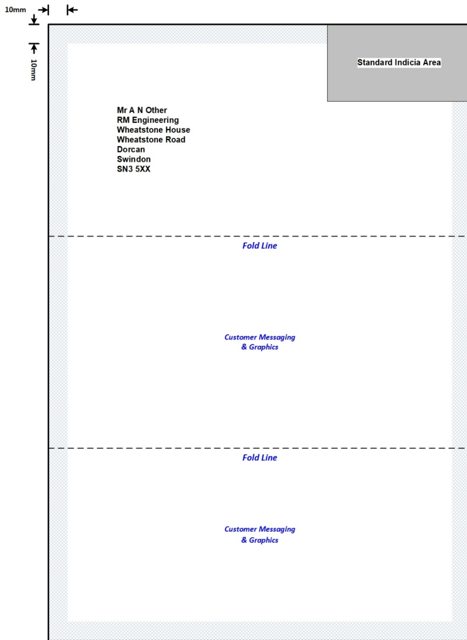
Figure 24 - Standard One-Piece Letter Mailer - Internal Perimeter Clear Zone (Not to Scale)
