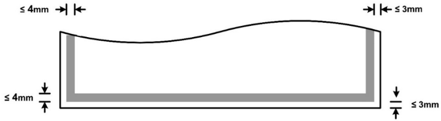
Figure 22 – Standard One-Piece Letter Mailer – Glue Line Requirements (Not to Scale)
