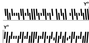
Figure 18 – 4-State Mailmark Barcode Bar Skew Y (Not to Scale)
