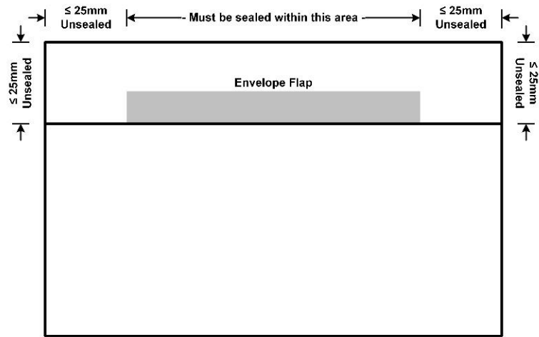
Figure 32 - Large Letter Sealing - Poly Envelope (Not to Scale)
