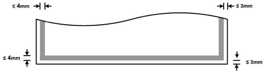
Figure 15 - Standard One-Piece Letter Mailer - Glue Line Requirements (Not to Scale)
