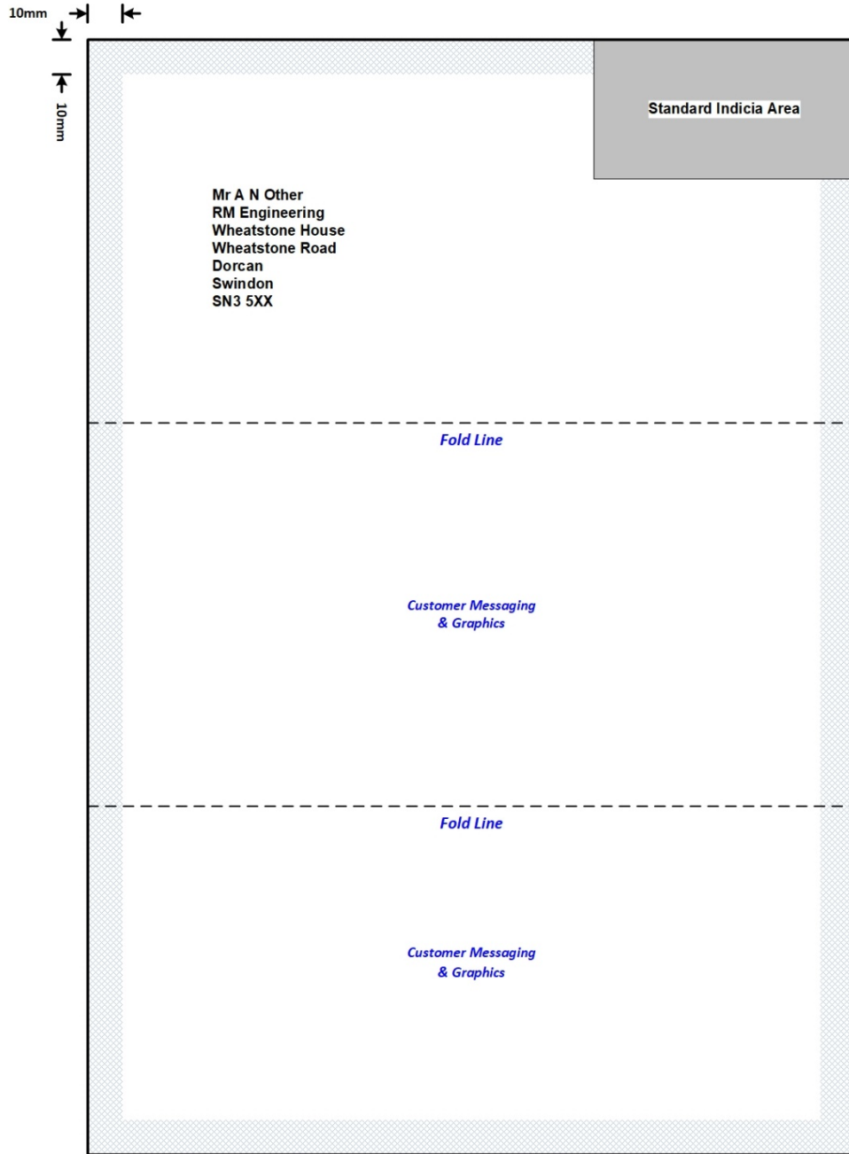
Figure 24 – Standard One-Piece Mailer - internal perimeter clear zone (not to scale)
