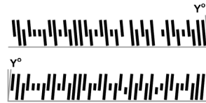
Figure 16 – 4-State Mailmark Barcode bar skew Y (not to scale)
