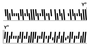
Figure 16 – 4-State Mailmark Barcode Bar Skew Y (Not to Scale)
