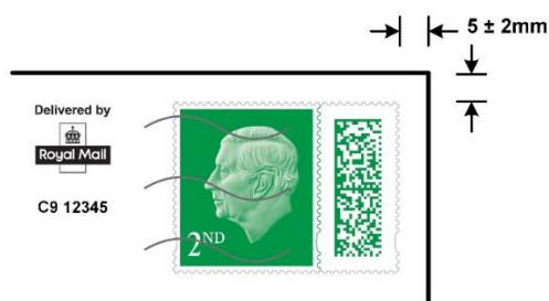
Figure 34: Digital Stamp Indicator layout and positioning
